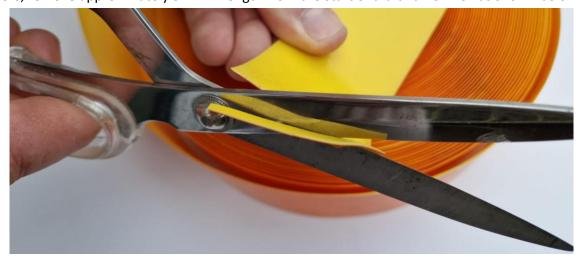
Slowly peel back part of the release liner. The liner should come away from the tape with ease leaving the adhesive membrane intact.
